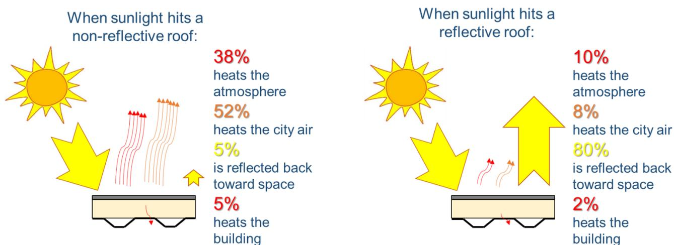
**Figure 2. Reflective versus Non-reflective Roof: Where Does the Heat Go?**
