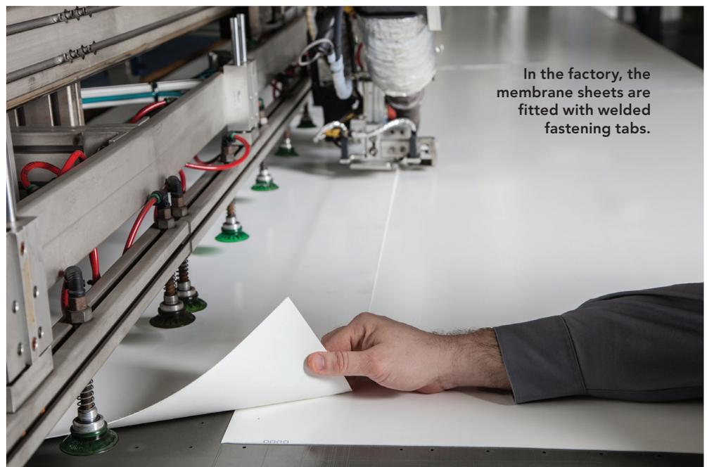
In the factory, the membrane sheets are fitted with welded fastening tabs.
