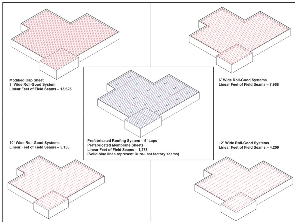
When the vast majority of the seaming for a prefabricated membrane is done in the factory, that leaves very little to do on the rooftop. When the entire roofing system is fabricated on the rooftop, the number of seams to weld on-site increases dramatically.
